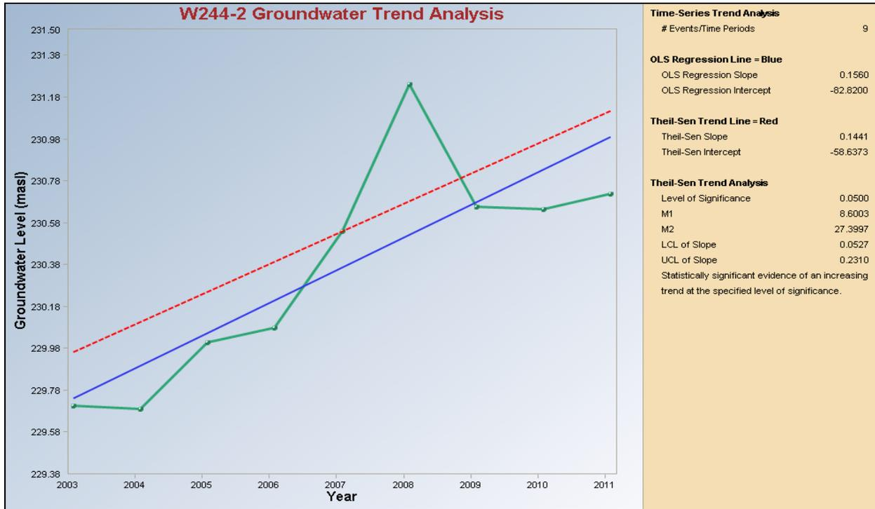
Figure 7: Illustration of results from Theil-Sen trend test for groundwater level data for W244-2 at 95% confidence coefficient.
