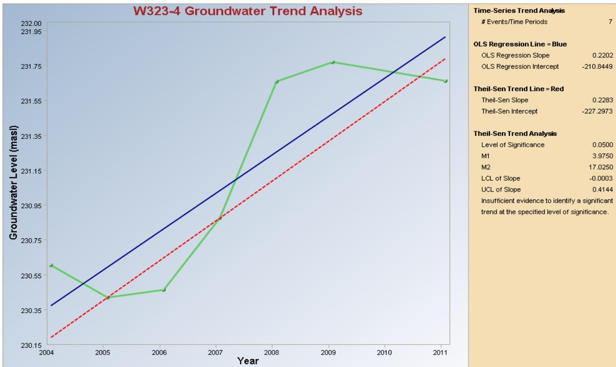
Figure 9: Illustration of results from Theil-Sen trend test for groundwater level data for W323-4 at 95% confidence coefficient.
