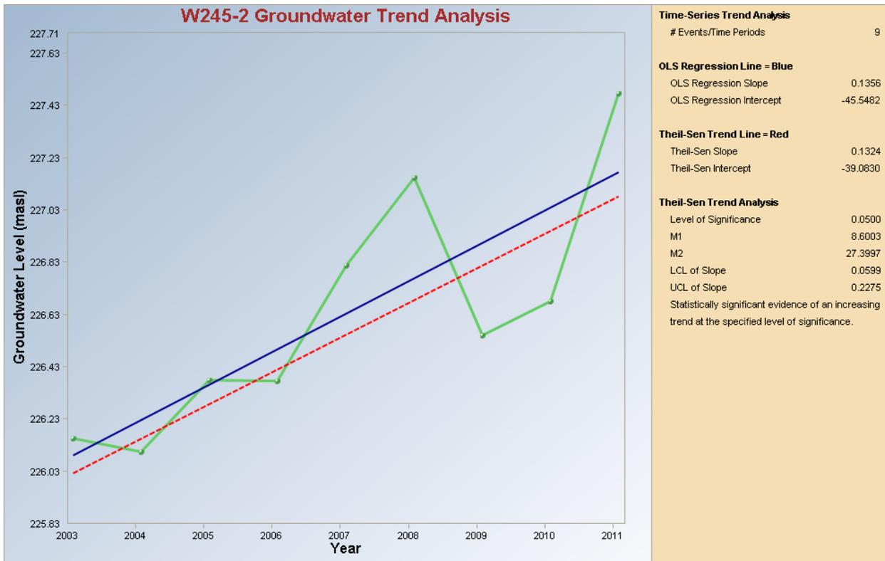
Figure 8: Illustration of results from Theil-Sen trend test for groundwater level data for W245-2 at 95% confidence coefficient.
