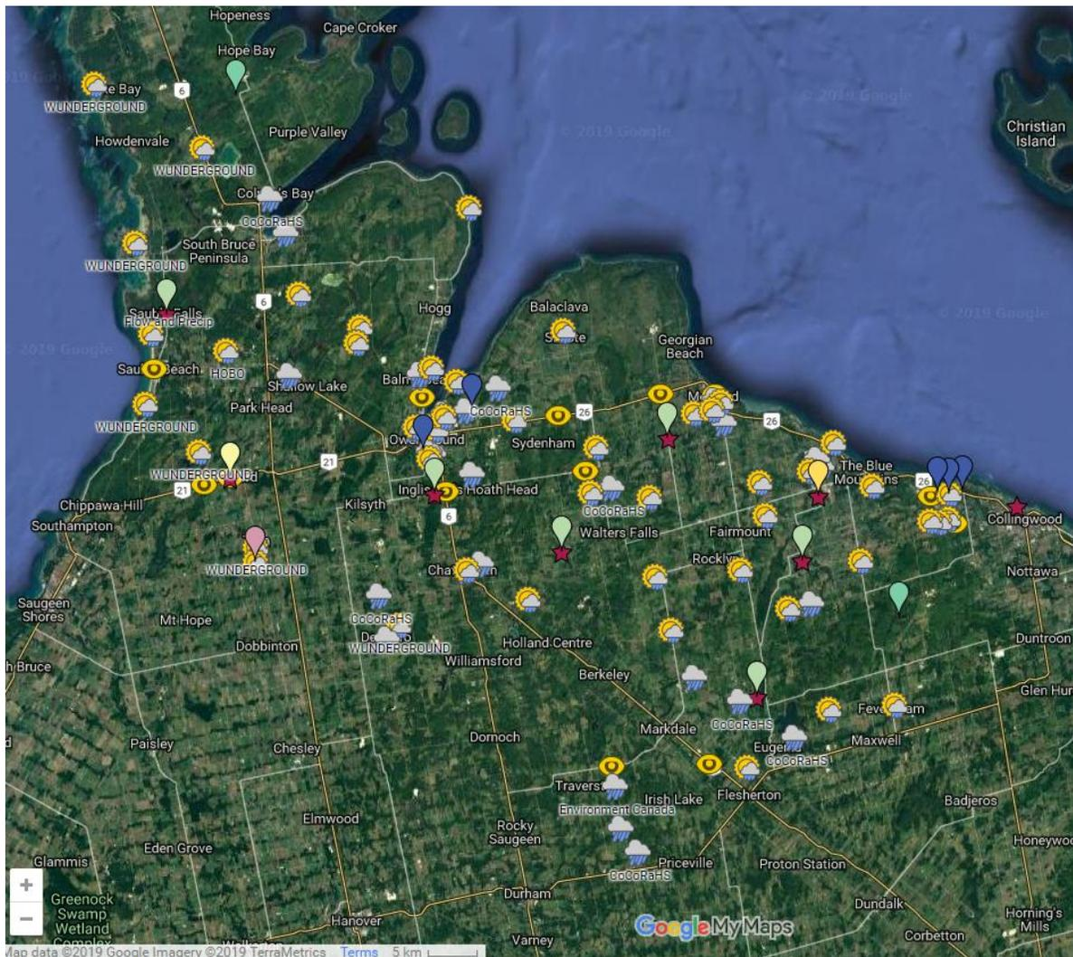
*Figure 3: Stream flow, precipitation and weather gauges, and weather cameras used by the GSCA (2019). Weather icons denote network type (rainy icon is either CoCoRaHS or ECCC; partial sun icon is Weather Underground, WeatherLink, or HOBO stations). Yellow eye icons denote weather cameras. Red star icons denote Water Survey of Canada flow gauges and the coloured map pins summarize the type of data available from flow gauges.*
