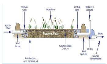
This sub-surface flow wetland can treat runoff from livestock yards or tile drains. Treatment wetlands for manure runoff can reduce Suspended Sediment, Biological Oxygen Demand, Phosphorus, Nitrogen and fecal bacteria by 80-90%
