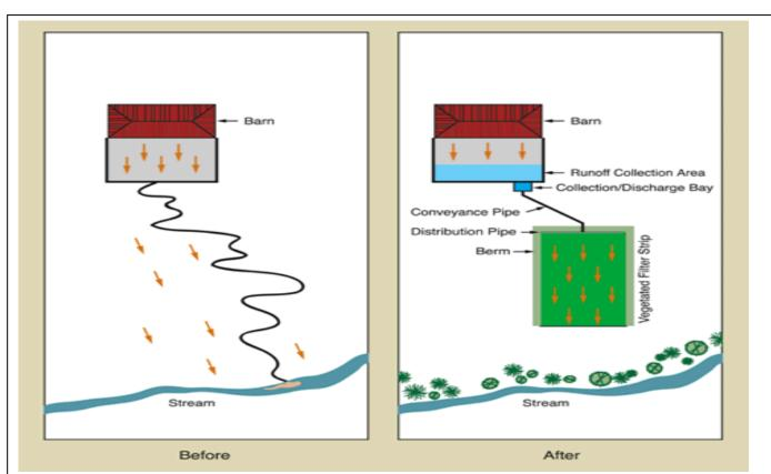
A manure runoff treatment system can significantly reduce the concentrations of bacteria, nitrogen, phosphorus and biochemical oxygen demand. Treatment systems consist of the following parts: runoff/contaminant reduction, runoff collection, delivery, and treatment area.
