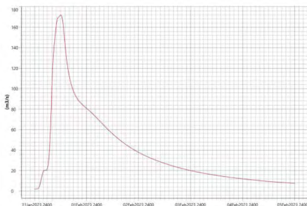
Figure 6-3. River: Mad River → Junction Jun-05 → Timmins Regional Max Peak Flow Q = 171.79 cms
